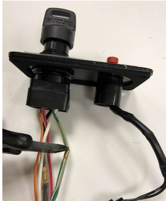
Key switch with one green wire
