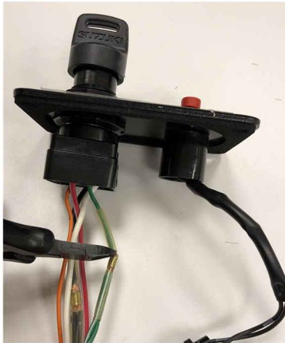
Key switch with one green wire
