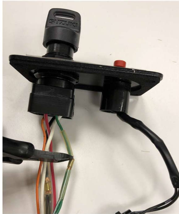
Key switch with one green wire
