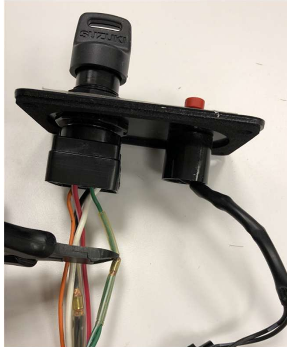
Key switch with one green wire
